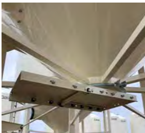
Adjustable Rack & Pinion Slide Gate Assembly. Available in Stainless Steel
